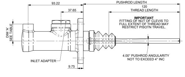
3/8" x 24 UNF OUTLET 104.30 AEROQUIP ADAPTER -BOOT SHOWN FULLY EXTENDED, ADJUST TO YOUR LIKING. **AVAILABLE** Ø36.00 Ø35.00 BOOT DIA 7/16" x 20 UNF INLET 9.5 97 84 Ø17.80 32.
